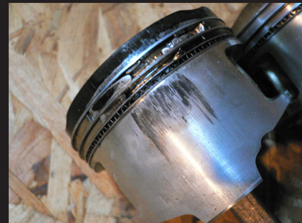
FIGURE 2 (LEFT) - PISTON WEAR DUE TO LACK OF LUBRICATIONS
