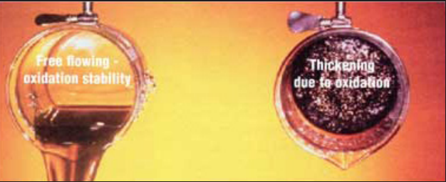
FIGURE 2 - ENGINE OIL OXIDATION • Left: Free flowing due to oxidation stability of oil • Right: Thickening due to oxidation of oil
