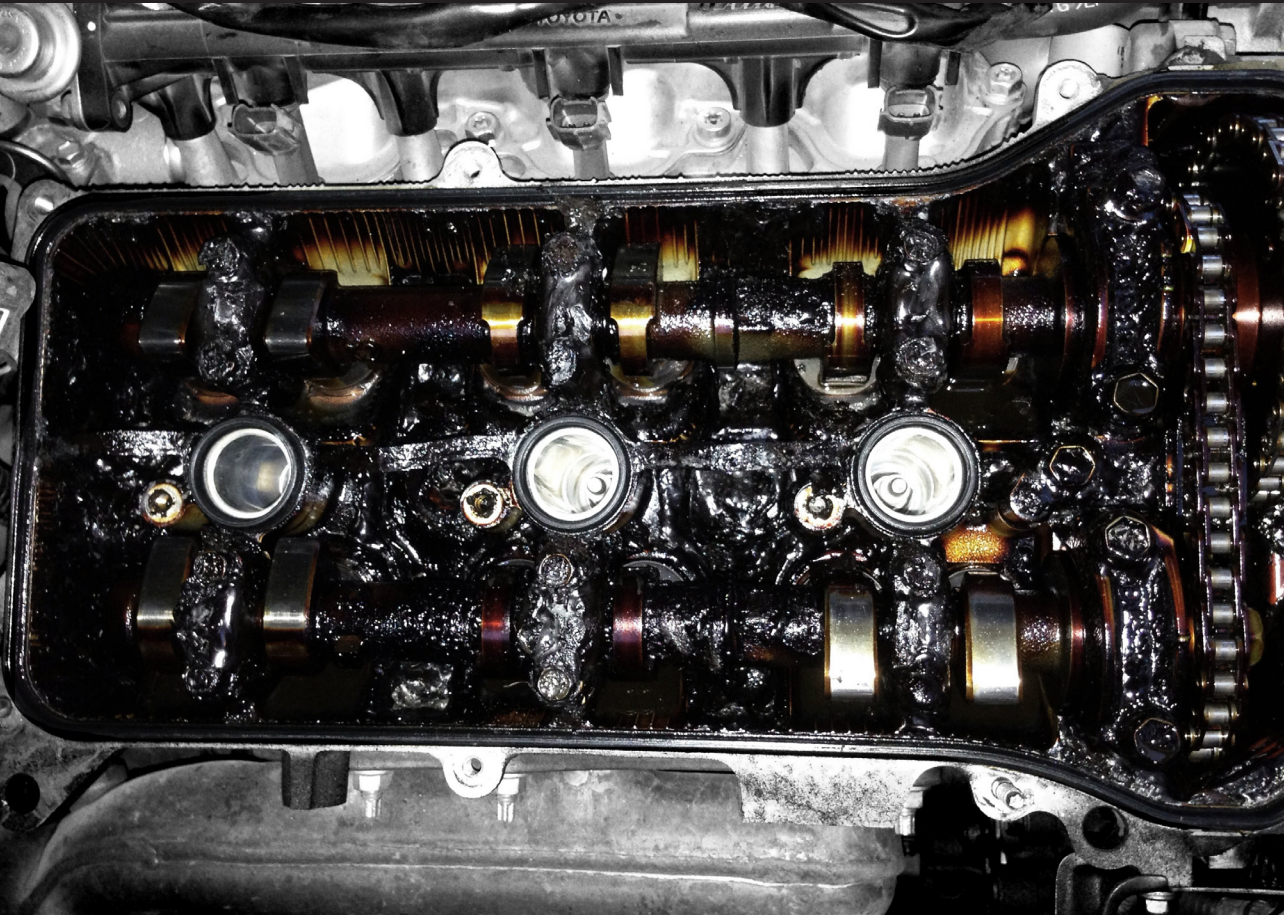
FIGURE 5 (UPPER) - TOP DECK (CYLINDER HEAD) SLUDGING • Heavy sludge buildup resulting from cold engine operation combined with an oil of inadequate quality
