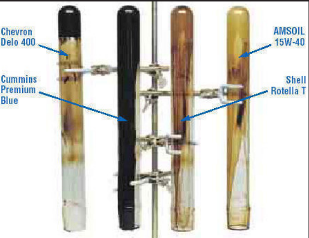
FIGURE 3 - THERMAL STABILITY OF OIL • From left to right: Solid deposits, Heavy deposits, Medium deposits and Very light deposits • The high temperature stability of engine oil keeps engine cleaner and performs longer
