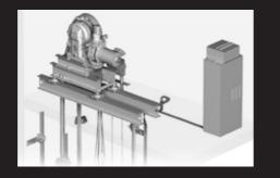
FIGURE 2 - TRACTION METHODS Upper: Geared · Lower: Gearless The typical viscosities of lubricants for elevator reduction gear systems are usually ISO320 and ISO460 (depends on the machine requirements and other environmental factors). The following table shows some examples of Steel Shield lubricants:
