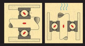
Axial or Thrust Load • When the load is parallel to the shaft • Left: Axial load in a horizontal pump gravity
