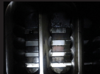
FIGURE 1 - PISTON RING INSPECTION FROM SCAVENGE PORT
