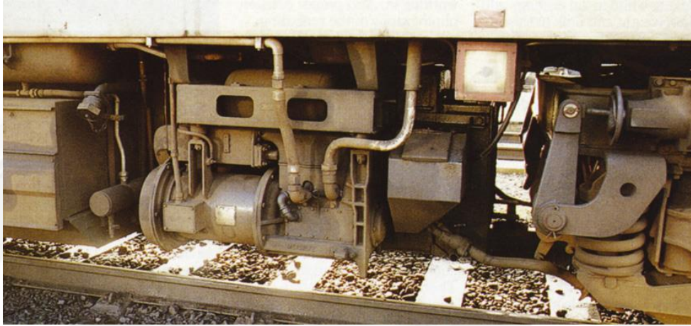
Air compressor with white pipes going to and from it
